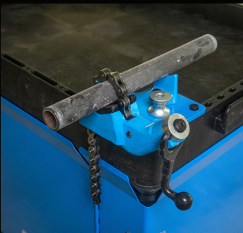
1/8" to 2-1/2" pipe capacity
